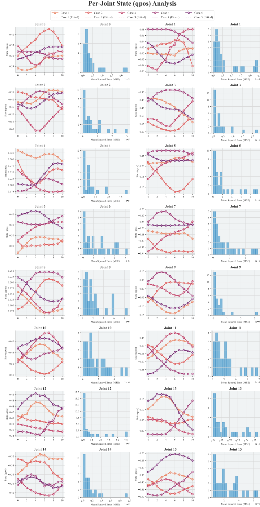
Figure 33: Polynomial Fitting (order = 5) and Error Distribution of Per-Joint State Sequences (window length = 10). In each group with two subfigures, the left one draws the original data sequence and the fitted sequence using a 5-ordered polynomial function while the right one shows the fitting error distribution.
